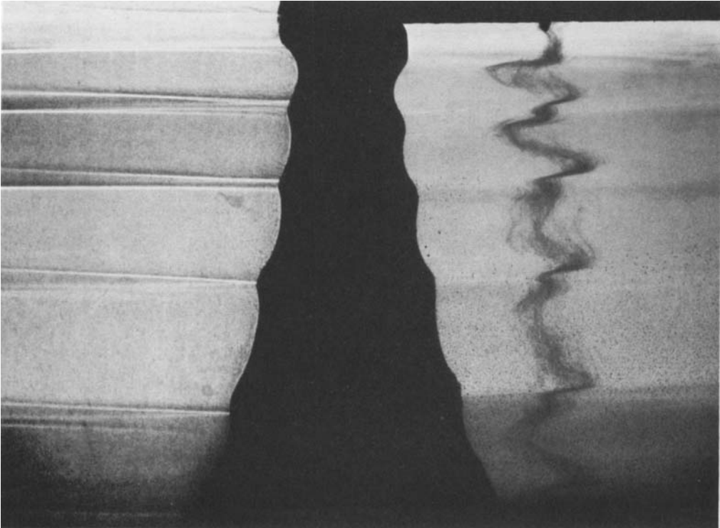
FIGURE 10. A crystal column produced by cooling an initially homogeneous solution of \text{Na}_2\text{CO}_3 at a central pipe. Upflow in the boundary layer due to crystallization has produced stratification and layering and associated 'scallops' on the crystal surface. The left of the picture is a shadowgraph and the right shows a dye streak against diffuse back lighting, with the distortions indicating the motion in the layers.
